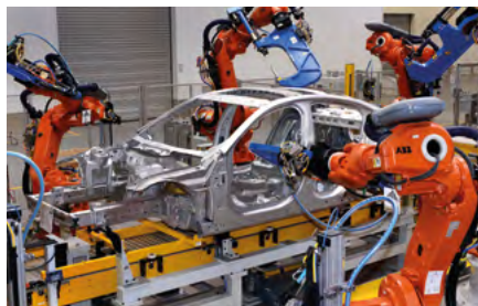
An aluminium body shell on our production line at Solihull.
